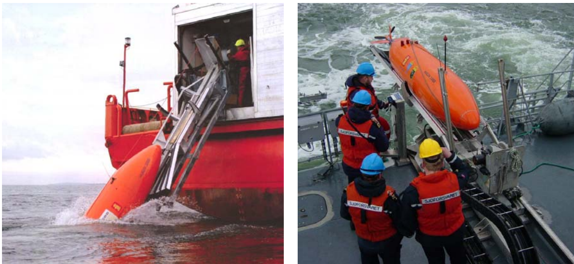
Figure 1: HUGIN AUVs. Left: A HUGIN 3000 vehicle operated by Fugro NV, the Netherlands; right: A HUGIN 1000 vehicle operated by RNoN from the mine hunter HNoMS Karmoy .
